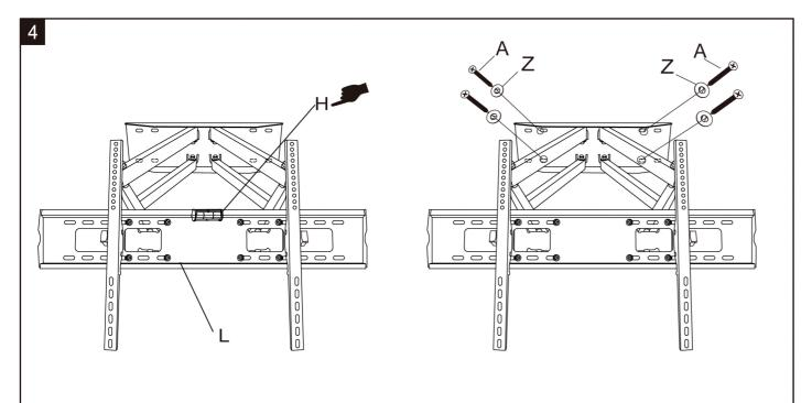
Position the wall plate so mounting holes line up with wall studs. Put level (H) on the top edge of the wall plate to make sure the wall plate is level. Attach wall plate to wall using screws (A) and washers (Z).
