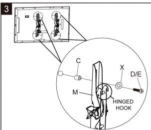
Place TV bracket, flat side down, on the back of the TV. The hinged hook must be towards the top. Place spacers (C) and washer (X) between the TV back and the TV bracket. Attach TV bracket to TV using either screws (D,E, depending on TV brand).
