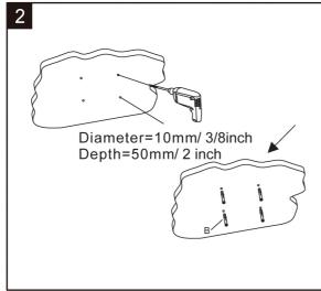
Put the plastic knob(G) on the hole of hooks,and tighten it with the Bolt(F). Use the wall plate template to determine the proper location to drill holes for the wall plate.Drill the determined holes on the wall, then put the 10×48 Anchor(B) in the holes.
